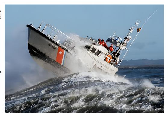
full of state-of-the-art technology. It is designed for rapid response in extreme ocean conditions. How extreme? Design specifications say 30 foot seas or 20 foot surf with 50 knot winds. With waters like that, a capsize is certainly possible. Not to worry, the boat is designed to self-right in 30 seconds. Good to know, and not an experience you will soon forget.
